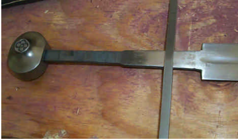
Figure 2: Del Tin 2142 Tang. Note sharp corners at change in cross section from blade and welded extension stub.
