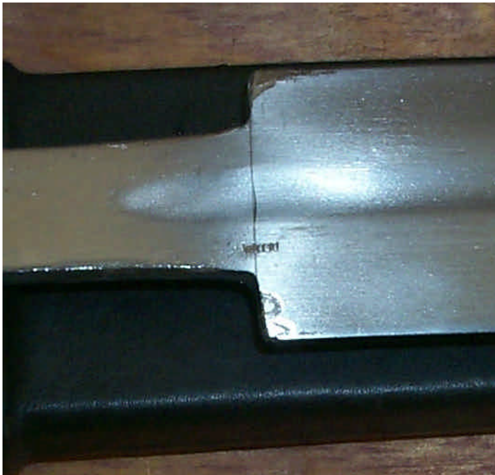
Figure 5: Gentle low temperature grinding removed old blade material and created rounded file transition to tang with taper to match hole in guard. This extended tang by 1/4" .
