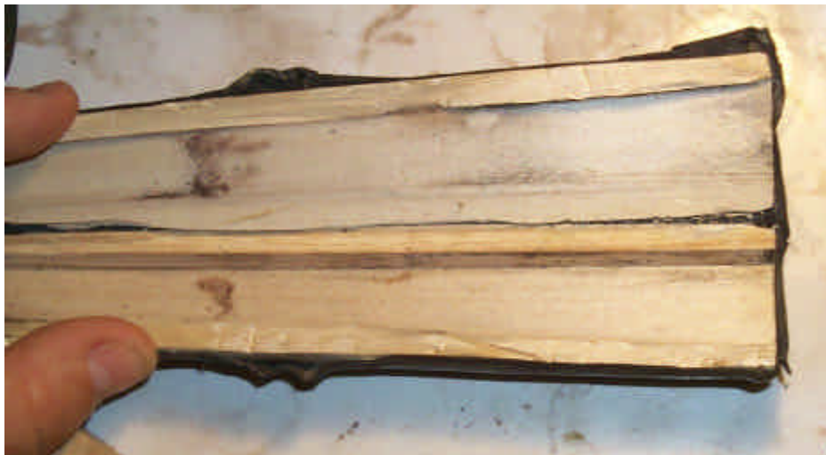
Figure 3: Tapered tang channel inside original soft wooden handle.
