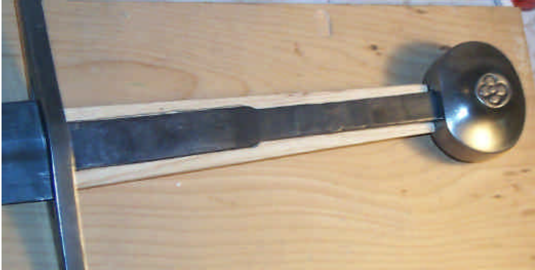
Figure 4: Custom fit of new handle to tang is snug.
