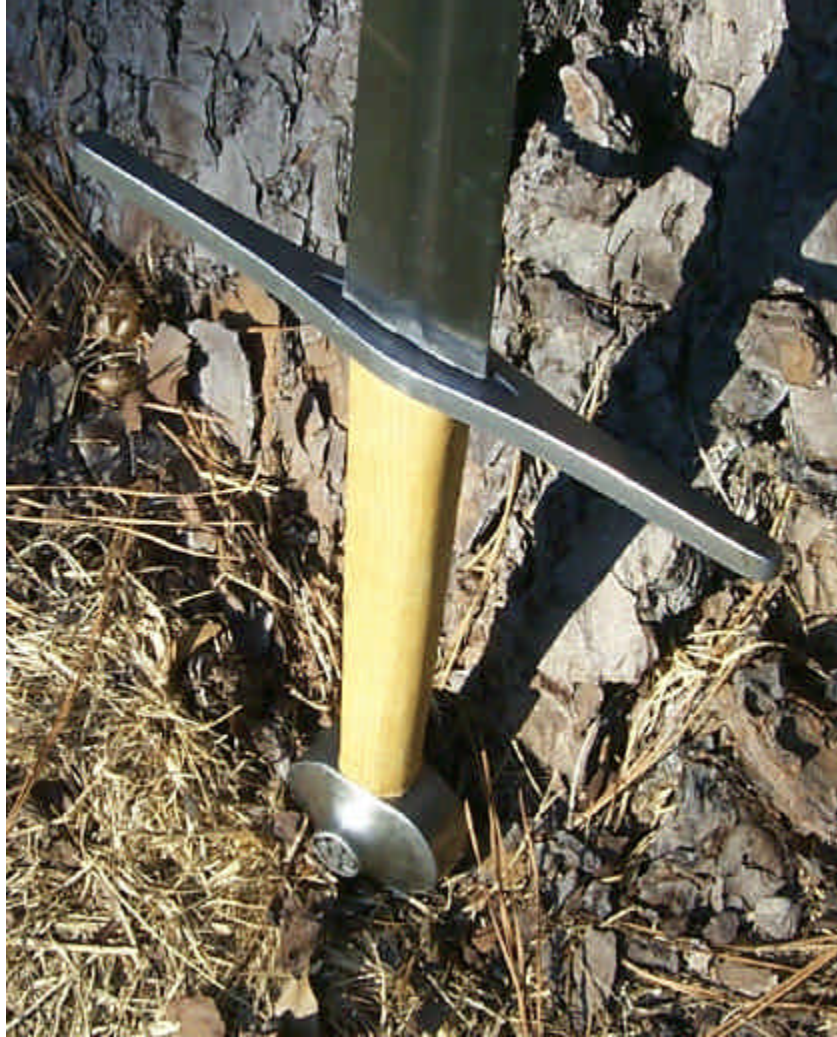
Figure 7: Liquid steel epoxy fills gaps in guard hole.
